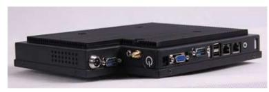
The industrial PC was developed specially for use in the POS area. Its super slim design and with its VESA-75 and VESA-100 holes on the front and a VESA-100 mount on the back it can be installed between an existing (Touch) Monitor (frontside)
